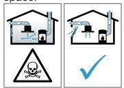
Always ensure adequate fresh air in the room if the appliance is being operated in exhaust air mode at the same time as a room-air-dependent heat-producing appliance is being operated.
