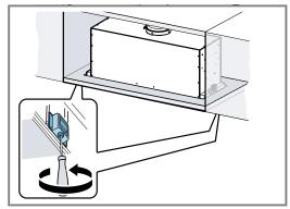
**3.** Screw in the front two screws and select a hole so that the surface of the appliance is flush with the fitted unit.
