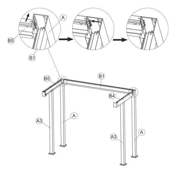
Connect the Leg Tube (A) and the Back Beam Tube (B1) to the Left Beam Tube (B5) and the Right Bean Tube (B4) as shown.
