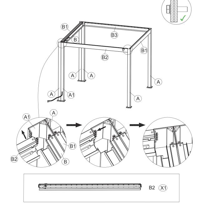
Attach the Right Beam Tube (B2) between the leg tubes (A) as shown. Align the connectors on the beam with the connection points on the leg tubes. Insert the screws into the connection points but leave them loose for adjustments. Ensure the correct screw orientation as indicated in the diagram.
