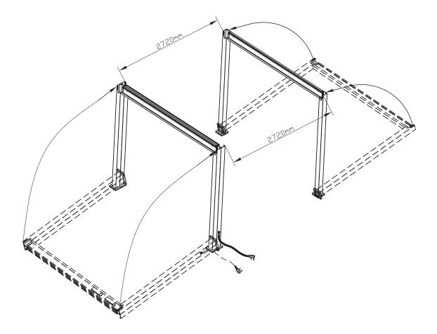
Carefully lift both assembled frame structures upright. Ensure the distance between the frames is 2720 mm as shown in the diagram. Adjust the frames to ensure they are properly aligned and level on the ground. Verify that all connections are still loose and ready for final adjustments before tightening.
