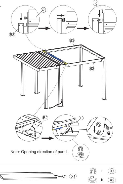
Insert a Light Louvre (C1) between the Right Beam Tube (B2) and Left Beam Tube (B3) and secure it as shown.
