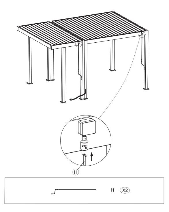
Insert the Rocker Handle (H) into the Turbo Motor as shown. Ensure the handle is securely in place and properly aligned for smooth manual operation of the louvre system.
