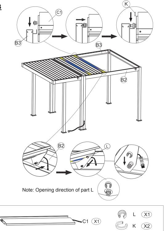
Insert a Light Louvre (C1) between the Right Beam Tube (B2) and Left Beam Tube (B3) and secure it as shown.
