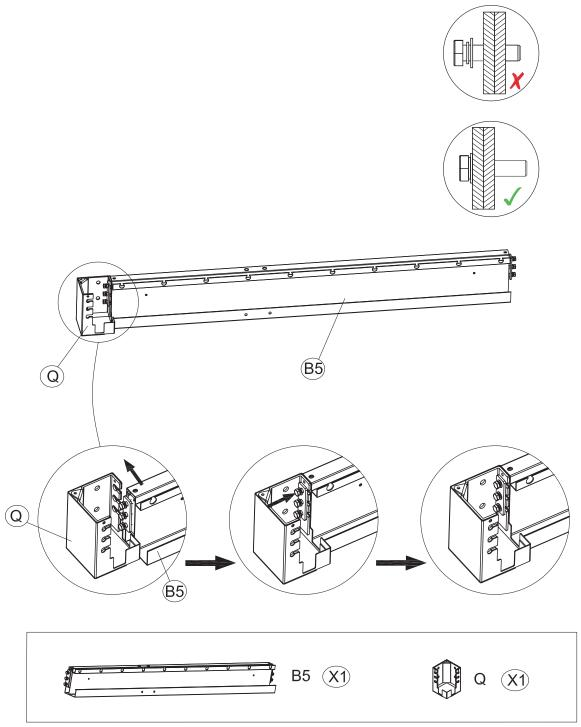
Attach the Beam Connector (Q) to the Left Beam Tube (B5) as shown. Align the connectors on the beam with the connection points on the leg tubes. Insert the screws into the connection points but leave them loose for adjustments. Ensure the correct screw orientation as indicated in the diagram.
