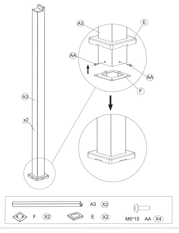
Slide the Footplate Cover 1 (E) over the base of Front Leg Tube (A3). Place the Footplate (F) right under the Front Leg Tube (A3). Use the M6\*15 Screws (AA) to secure the footplate and cover to the leg. Leave screws loose for now; tighten later.
