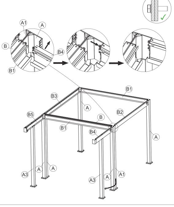
Attach the Right Beam Tube (B4) to the leg tubes (A) as shown. Align the connectors on the beam with the connection points on the leg tubes. Insert the screws into the connection points but leave them loose for adjustments. Ensure the correct screw orientation as indicated in the diagram.
