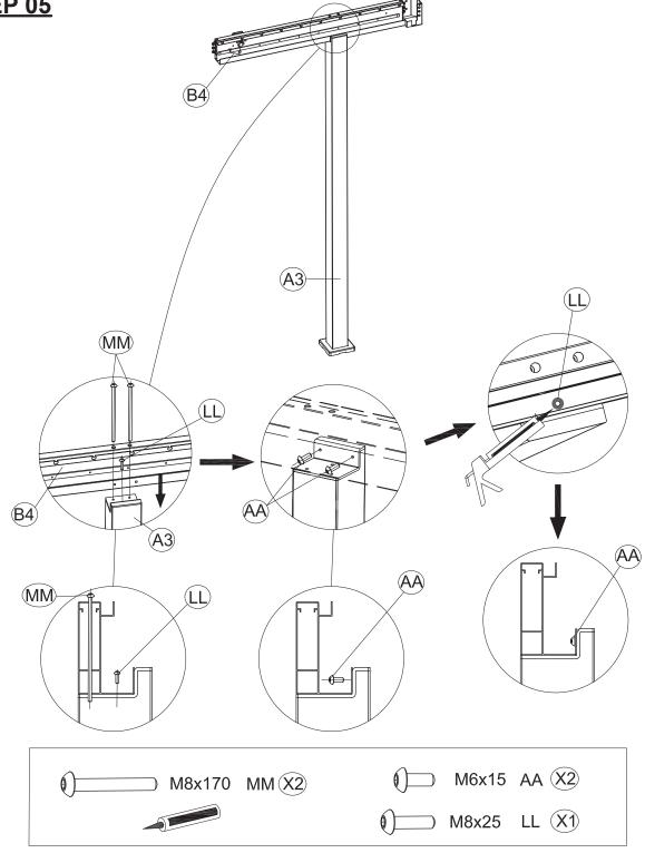
Connect the Right Beam Tube (B4) with Front Leg Tube (A3) as shown. Insert the screws (AA&LL&MM) into different screw holes as shown. Apply silicone neutral glass glue (not provided) along the screw LL as shown in the diagram. Ensure an even application of the glue to prevent any potential leaks. Note: glue is needed here to prevent water leakage
