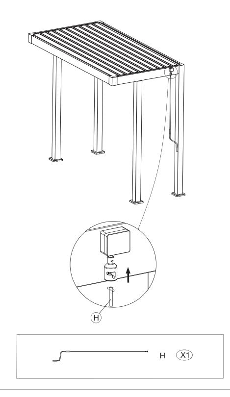
Insert the Rocker Handle (H) into the Turbo Motor as shown.
