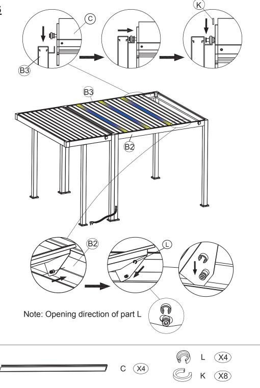
Insert 4 Louvres (C) between the Right Beam Tube (B2) and Left Beam Tube (B3) and secure it as shown.
