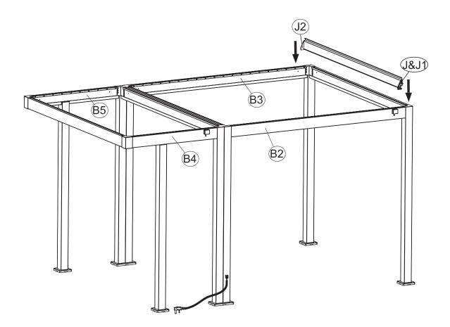
Position the Louvres (C) including the Light Louvres (C1) above the Beam Tubes (B2&B3, B4&B5) as shown.
