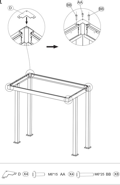
Attach the Cover for Leg Tube (D) to each corner of the structure, placing one cover on each corner.
