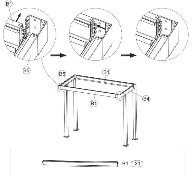
Connect another Back Beam Tube (B1) to the Left Beam Tube (B5) and the Right Bean Tube (B4) as shown.
