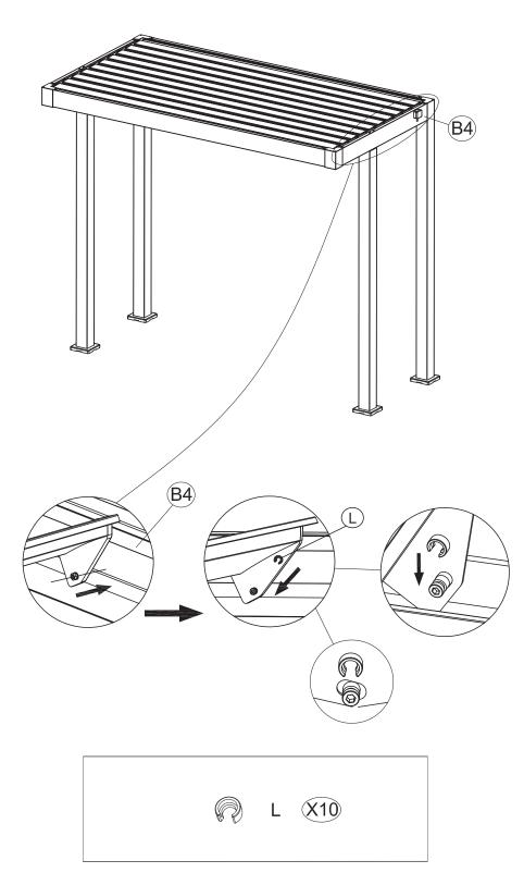
Install the Part L locks on the Right Beam Tube (B4) as indicated in the diagram, making sure the opening direction is comect. Tighten all the components securely.
