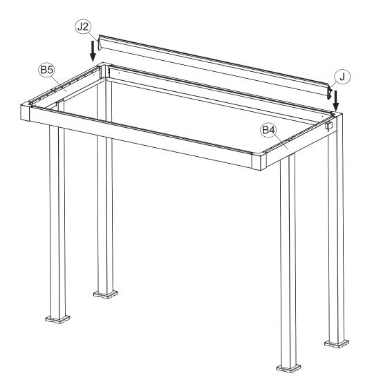
Position the Louvres (C) above the Right Beam Tube (B4) and Left Beam Tube (B5) as shown. Ensure the ends of louvres with Right Louvre Cap (J) are position on the Right Beam Tube (B4), the ends of louvres with Left Louvre Cap (J2) are position on the Left Beam Tube (B5). Ensure the louvres are correctly aligned with the frame.
