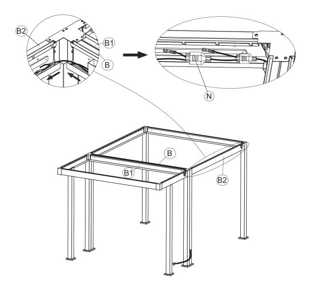
Straighten Part N (the wiring) to ensure it is properly aligned. Place Part N into the drain slot located on Right Beam Tube (B2) as shown in the diagram.
