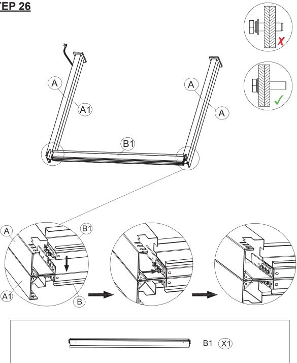
Connect the Front Beam Tube (B1) to Leg Tube1 (A) and Leg Tube 2 (A1). Align the connectors as shown in the diagram, ensuring the wiring from Leg Tube 2 (A1) is properly positioned.
