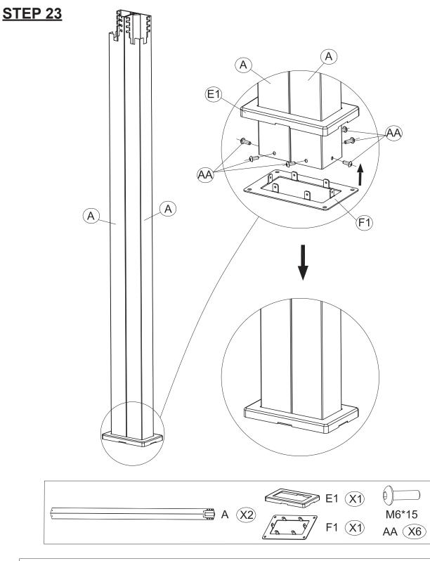
Align two Leg Tubes (A) together. Slide the Footplate Cover 2 (E1) over the base of two Leg Tubes (A). Place the Footplate 2 (F1) right under two Leg Tubes (A). Use the M6\*15 Screws (AA) to secure the footplate and cover to the leg. Leave screws loose for now; tighten later.
