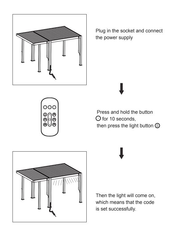
The code setting is only necessary when using the product for the first time, or after changing the remote control.
