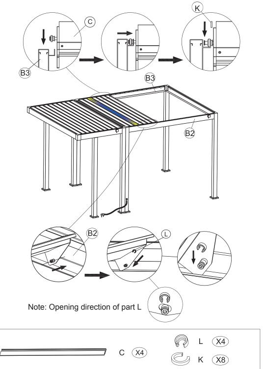
Insert 4 Louvres (C) between the Right Beam Tube (B2) and Left Beam Tube (B3) and secure it as shown.
