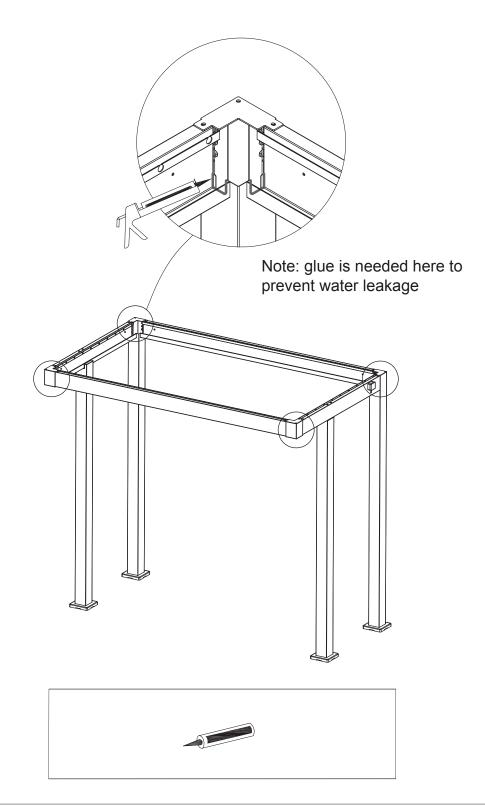
Apply silicone neutral glass glue (not provided) along the indicated seams in the corner joints as shown in the diagram.
