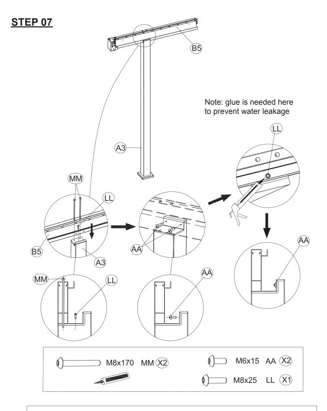
Connect the Left Beam Tube (B5) with Front Leg Tube (A3) as shown. Insert the screws (AA&LL&MM) into different screw holes as shown. Apply silicone neutral glass glue (not provided) along the screw (LL) as shown. Ensure an even application of the glue to prevent any potential leaks.
