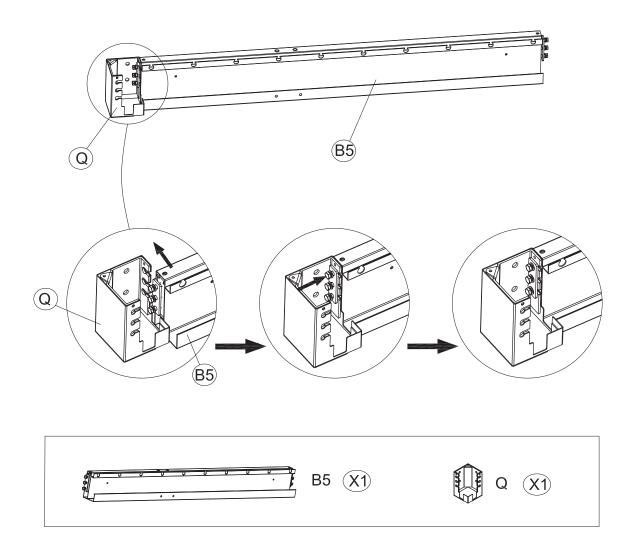
Connect the Beam Connector (Q) to the Left Beam Tube (B5) as shown. Ensure the connector is properly slotted into the beam, aligning securely. Tighten the screws, but leave them slightly loose for adjustments. Ensure the correct screw orientation, with the bolt fully inserted, as indicated in the diagram.
