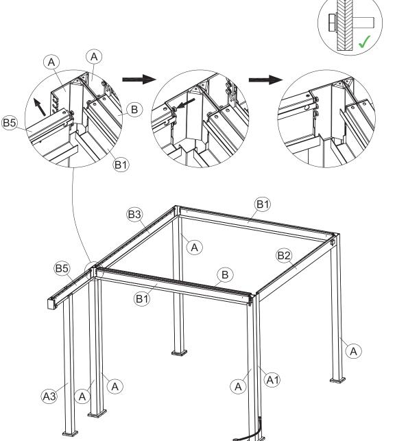
Attach the Left Beam Tube (B5) to the leg tubes (A) as shown. Align the connectors on the beam with the connection points on the leg tubes. Insert the screws into the connection points but leave them loose for adjustments. Ensure the correct screw orientation as indicated in the diagram.
