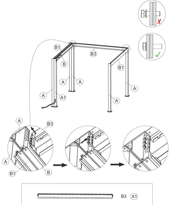
Attach the Left Beam Tube (B3) between the leg tubes (A) as shown. Align the connectors on the beam with the connection points on the leg tubes. Insert the screws into the connection points but leave them loose for adjustments. Ensure the correct screw orientation as indicated in the diagram.
