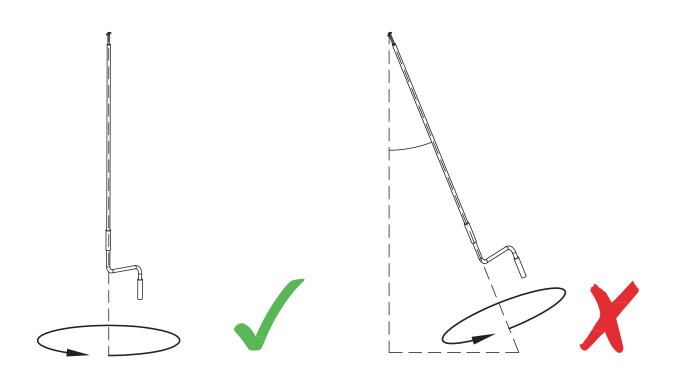
3. To open the louvre, turn the rocker handle clockwise; to close the louvre, turn the rocker handle anti-clockwise.
