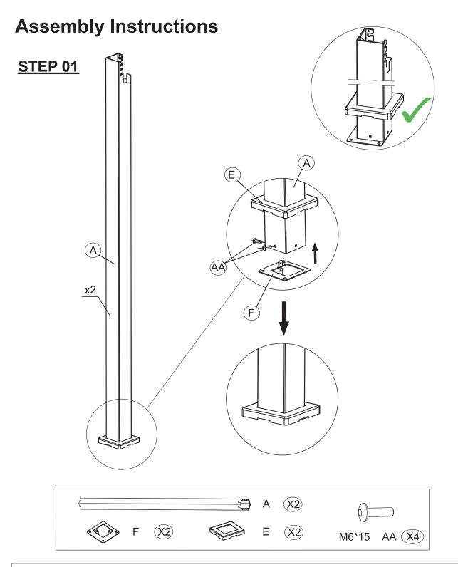
Slide the Footplate Cover 1 (E) over the base of Leg Tube (A).
