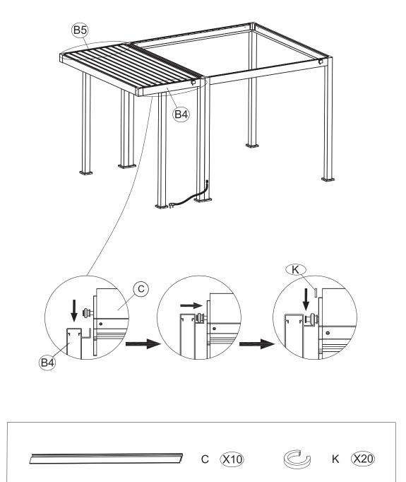
Insert 10 Louvres (C) between the Right Beam Tube (B4) and Left Beam Tube (B5) and secure it as shown.
