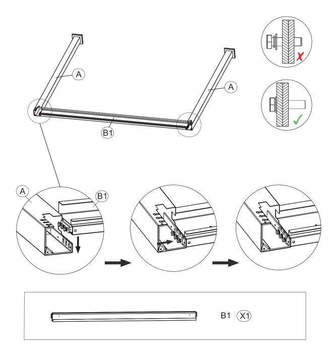
Connect the Front Beam Tube (B1) to Leg Tube 1 (A) as shown. Ensure the beam is properly slotted into the leg, aligning the connectors securely. Tighten the screws, but leave them slightly loose for adjustments. Ensure the correct screw orientation, with the bolt fully inserted, as indicated in the diagram.
