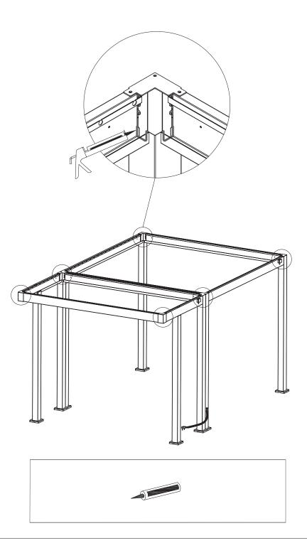
Apply silicone neutral glass glue (not provided) along the indicated seams in the corner joints as shown in the diagram.
