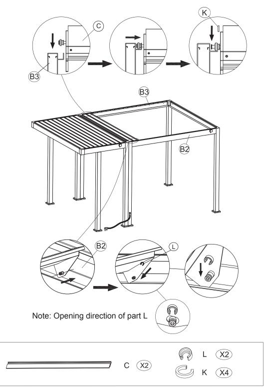
Insert 2 Louvres (C) between the Right Beam Tube (B2) and Left Beam Tube (B3) and secure it as shown.
