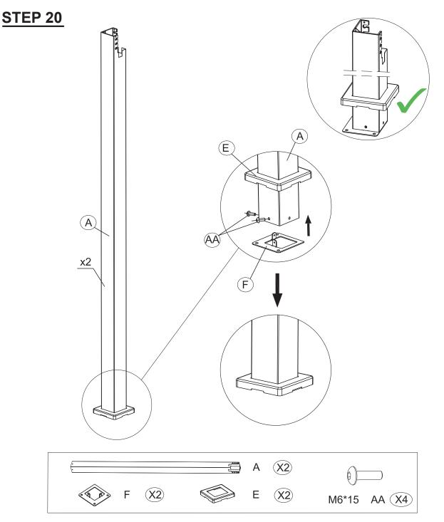
Slide the Footplate Cover 1 (E) over the base of Leg Tube 1 (A).
