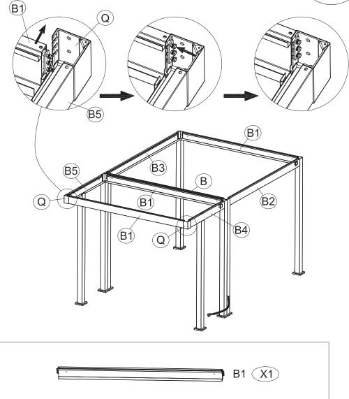
Attach the Back Beam Tube (B1) to two Beam Connectors (Q) as shown. Align the connectors on the beam with the connection points on the leg tubes. Insert the screws into the connection points but leave them loose for adjustments. Ensure the correct screw orientation as indicated in the diagram.
