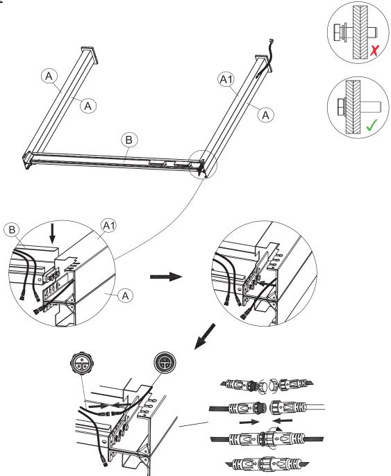
Connect the Front Beam Tube (B) to Leg Tube1 (A) and Leg Tube 2 (A1).
