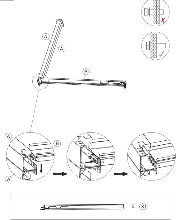
Connect the Front Beam Tube (B) to Leg Tube 1 (A) as shown.
