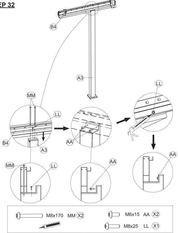
Connect the Right Beam Tube (B4) with Front Leg Tube (A3) as shown. Insert the screws (AA&LL&MM) into different screw holes as shown. Apply silicone neutral glass glue (not provided) along the screw LL as shown in the diagram. Ensure an even application of the glue to prevent any potential leaks. Note: Glue is required here to prevent leaks.
