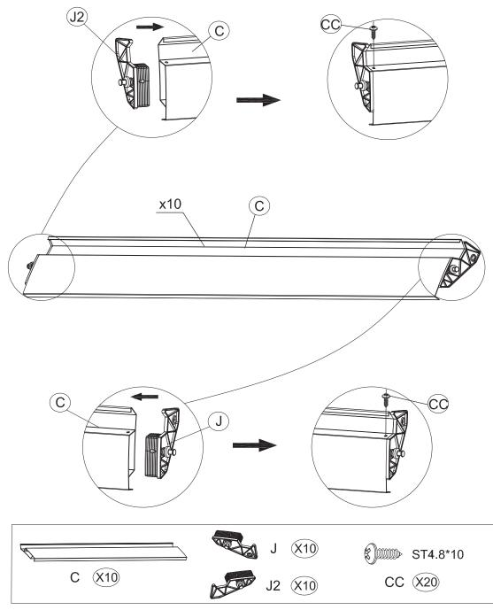
Attach the brackets (J2) and (J) to the Louvre (C) on both sides of the frame as shown in the diagram.
