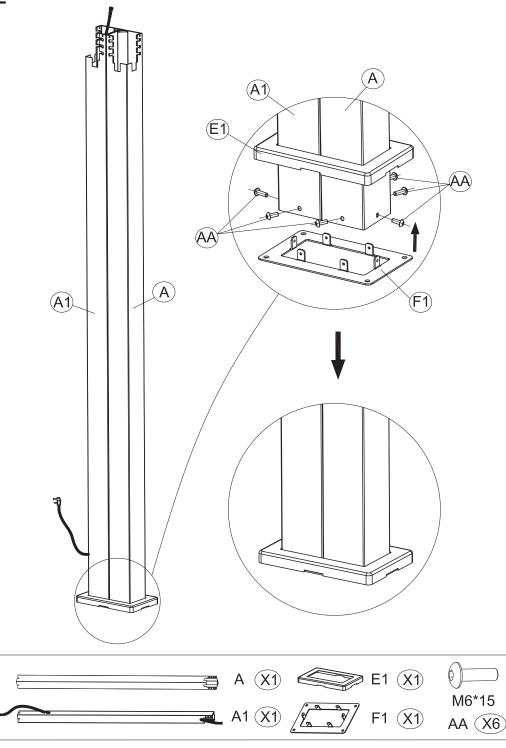
Align the Leg Tube (A) and the Leg Tube 1 (A1) together. Slide the Footplate Cover 2 (E1) over the base of two Leg Tubes (A&A1). Place the Footplate 2 (F1) right under two Leg Tubes (A&A1). Use the M6\*15 Screws (AA) to secure the footplate and cover to the leg. Leave screws loose for now; tighten later.
