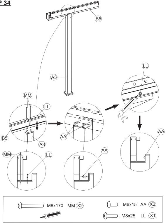
Connect the Left Beam Tube (B5) with Front Leg Tube (A3) as shown. Insert the screws (AA&LL&MM) into different screw holes as shown. Apply silicone neutral glass glue (not provided) along the screw LL as shown in the diagram. Ensure an even application of the glue to prevent any potential leaks. Note: Glue is required here to prevent leaks.
