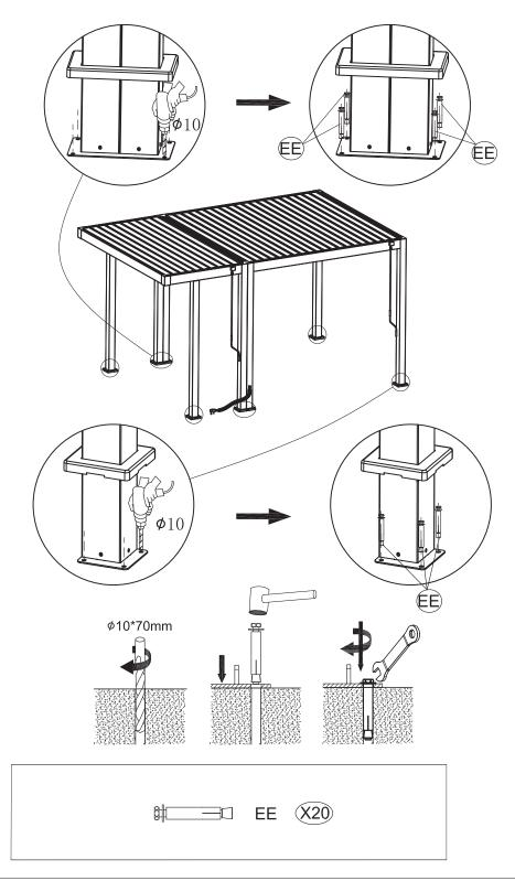
Drill holes into the ground using a 10 mm drill bit to a depth of 70 mm at the locations where the legs will be anchored.
