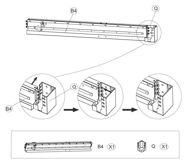
Attach the Beam Connector (Q) to the Right Beam Tube (B4) as shown. Align the connectors on the beam with the connection points on the leg tubes. Insert the screws into the connection points but leave them loose for adjustments. Ensure the correct screw orientation as indicated in the diagram.
