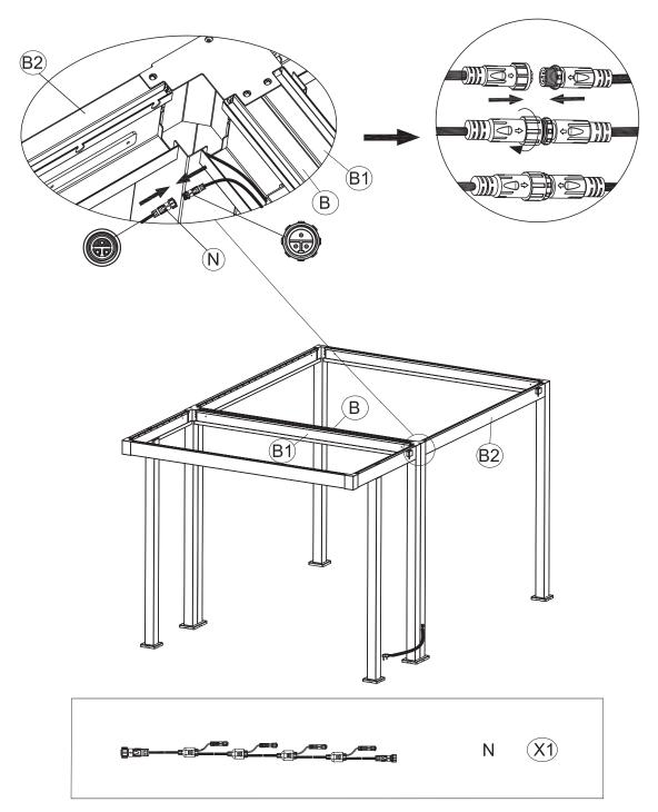
Insert Part N (wiring) into the designated connection points located at Front Beam Tube (B) as shown in the diagram.
