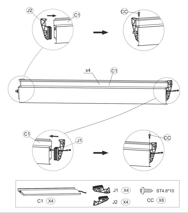
Attach the Light Louvre (C1) to the brackets (J2) and (J1) on both sides of the frame as shown. Insert the Louvre Cap without Hole (J2) into one side and the Louvre Cap with Hole (J1) into the other side for each light louvre.
