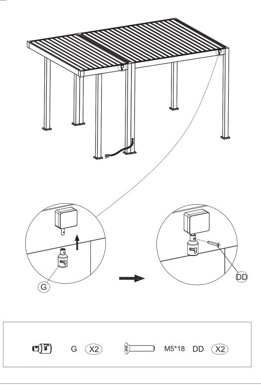
Attach Turbo Motor (G) to the designated area on the structure as shown. Secure the motor using the M5\*18 Screw (DD). Ensure the motor is properly fastened and aligned for smooth operation.
