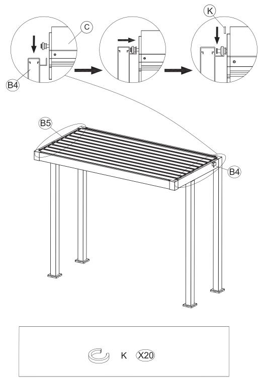
Insert all Louvres (C) between Right Beam Tube (B4) and Left Beam Tube (B5) and secure it as shown.
