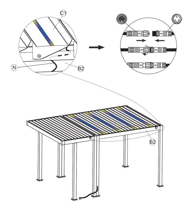
Locate the wiring Part N and ensure it is properly aligned with the connectors inside the Right Beam Tube (B2).
