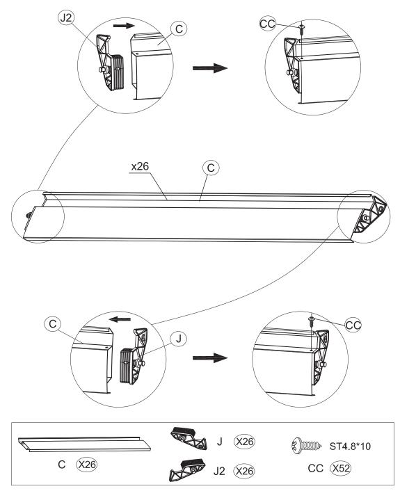
Attach the Louvre (C) to the brackets (J2) and (J) on both sides of the frame as shown in the diagram.
