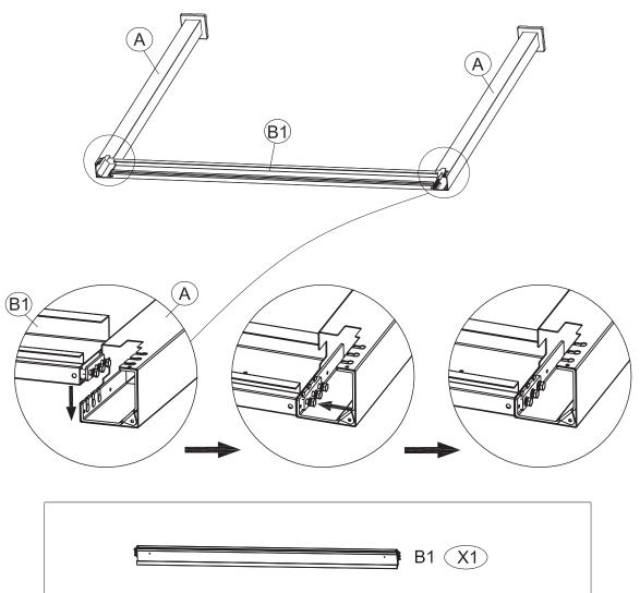
Connect the Back Beam Tube (B1) to Leg tube (A) as shown. Ensure the beam is properly slotted into the leg, aligning the connectors securely. Tighten the screws, but leave them slightly loose for adjustments. Ensure the correct screw orientation, with the bolt fully inserted, as indicated in the diagram.
