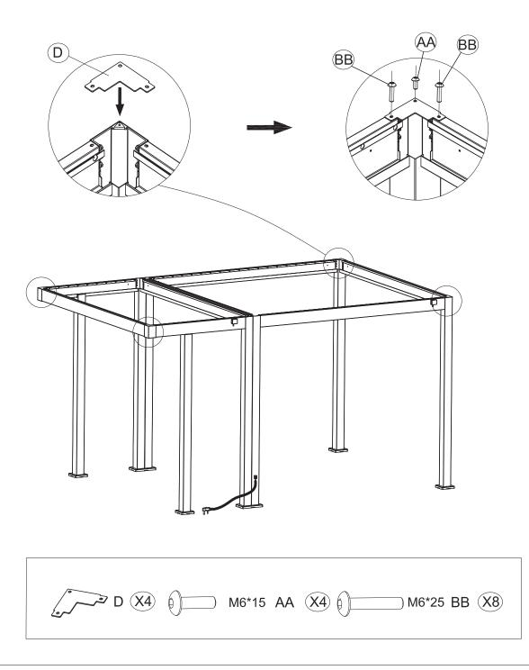
Attach the Cover for Leg Tube (D) to four corners of the structure as shown, placing one cover on each corner.
