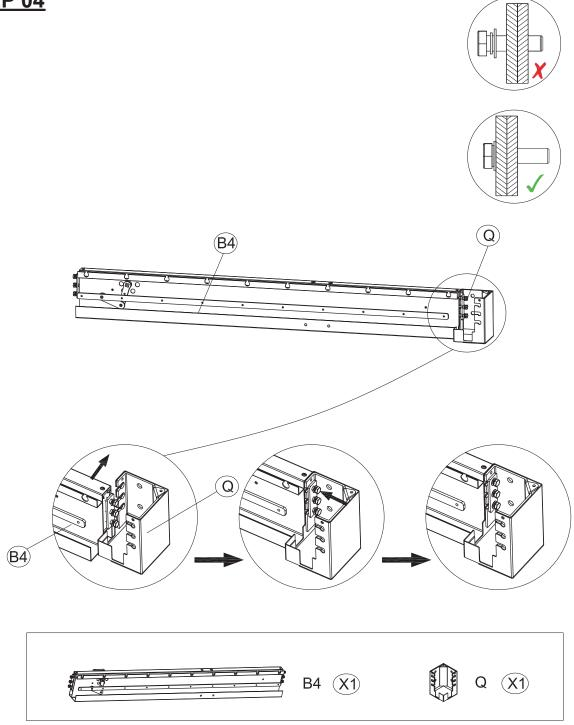
Connect the Beam Connector (Q) to the Right Beam Tube (B4) as shown. Ensure the connector is properly slotted into the beam, aligning securely. Tighten the screws, but leave them slightly loose for adjustments. Ensure the correct screw orientation, with the bolt fully inserted, as indicated in the diagram.
