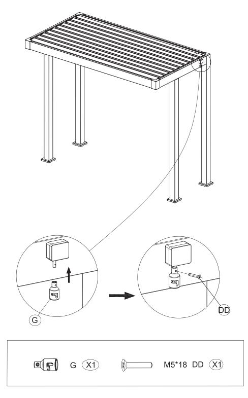
Attach Turbo Motor (G) to the designated area on the structure as shown. Secure the motor using the M5\*18 Screw (DD).
