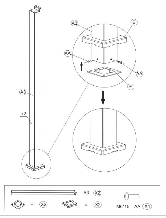
Slide the Footplate Cover 1 (E) over the base of Front Leg Tube (A3). Place the Footplate (F) right under the Front Leg Tube (A3). Ensure the directions of the Footplate (F) and the Front Leg Tube (A3) are the same as shown. Use the M6\*15 Screws (AA) to secure the footplate and cover to the leg. Leave screws loose for now; tighten later.
