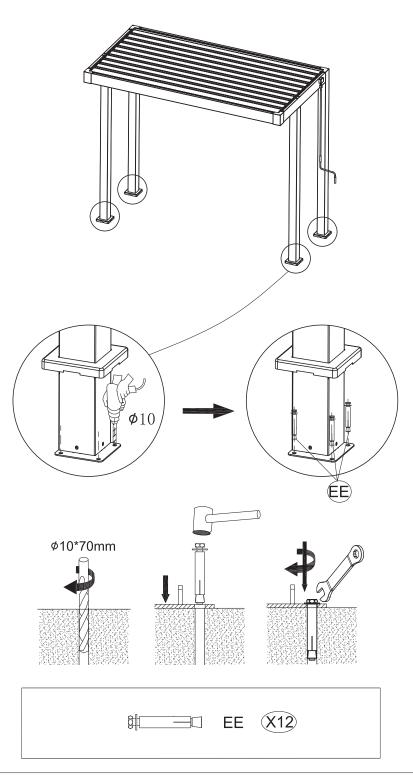
Drill holes into the ground using a 10 mm drill bit to a depth of 70 mm at the locations where the legs will be anchored.
