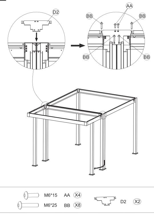
Attach the Cover for Leg Tube 1 (D2) to two connected corner of the structure as shown, placing one cover on each corner.
