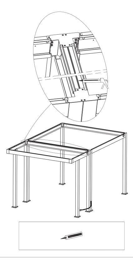
Apply silicone neutral glass glue (not provided) along the indicated seams in the corner joints as shown in the diagram.
