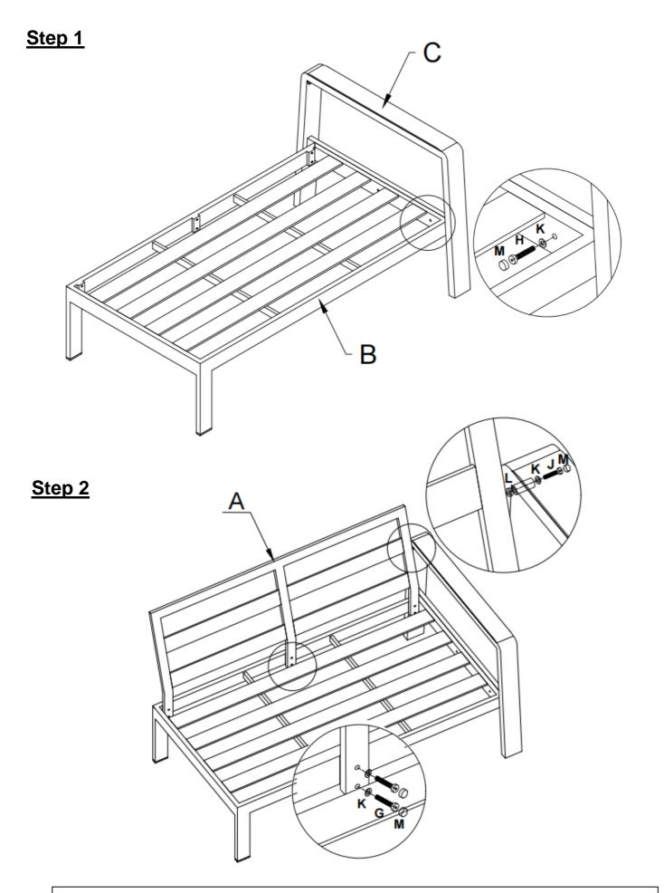
PLEASE ENSURE ALL FIXINGS ARE LEFT LOOSE DURING ASSEMBLY BUT ARE SECURELY TIGHTENED UPON COMPLETION.
