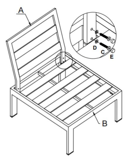
PLEASE ENSURE ALL FIXINGS ARE LEFT LOOSE DURING ASSEMBLY BUT ARE SECURELY TIGHTENED UPON COMPLETION.
