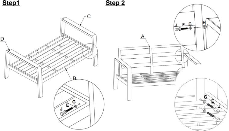
PLEASE ENSURE ALL FIXINGS ARE LEFT LOOSE DURING ASSEMBLY BUT ARE SECURELY TIGHTENED UPON COMPLETION.
