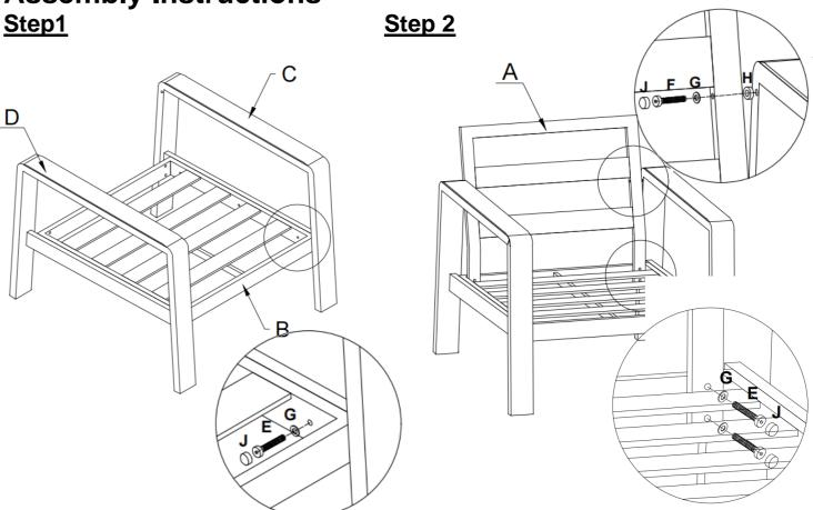
PLEASE ENSURE ALL FIXINGS ARE LEFT LOOSE DURING ASSEMBLY BUT ARE SECURELY TIGHTENED UPON COMPLETION.
