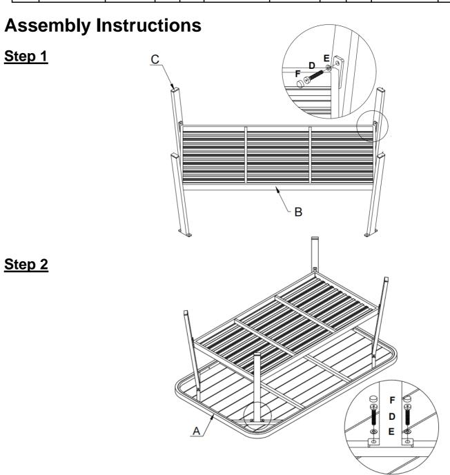
PLEASE ENSURE ALL FIXINGS ARE LEFT LOOSE DURING ASSEMBLY BUT ARE SECURELY TIGHTENED UPON COMPLETION.
