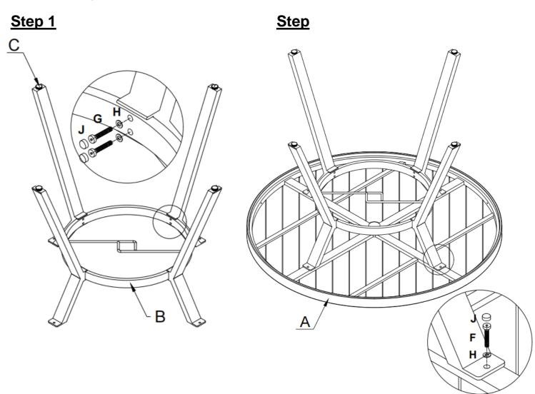
PLEASE ENSURE ALL FIXINGS ARE LEFT LOOSE DURING ASSEMBLY BUT ARE SECURELY TIGHTENED UPON COMPLETION.
