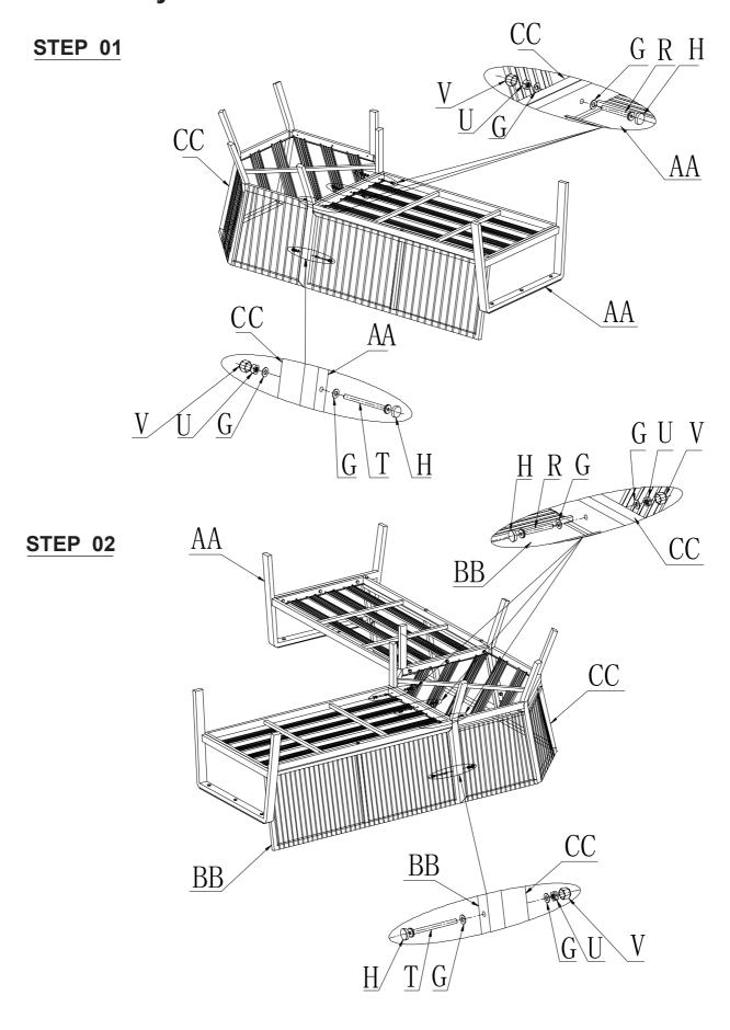
PLEASE ENSURE ALL FIXINGS ARE LEFT LOOSE DURING ASSEMBLY BUT ARE SECURELY TIGHTENED UPON COMPLETION.
