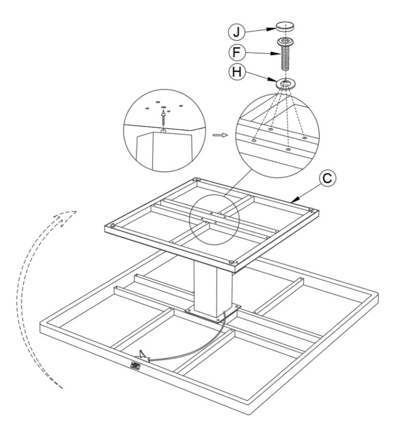
PLEASE ENSURE ALL FIXINGS ARE LEFT LOOSE DURING ASSEMBLY BUT ARE SECURELY TIGHTENED UPON COMPLETION.
