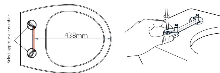
Once secured in place, remeasure the 438mm to check and remove the template. Attach the cover cap over each anchor and then click the seat in place.
