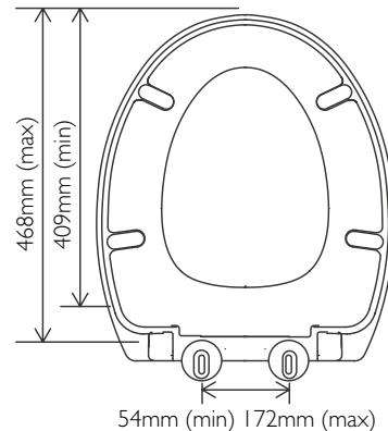
To install this toilet seat you will need fixing pack (provided) and phillips head screw driver. Do not use a battery driver or drill to assemble the toilet seat to the WC.
