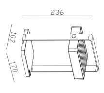
Voltage (V): 5 Volt IP degree: IP44 Class (Class 1, Class 2, Class 3): Class 3 (12V) Socket type: LED Module Switch placement: On the fixture
