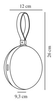
IP degree: IP54 Class (Class 1, Class 2, Class 3): Class 3 (12V) Socket type: LED Module Switch placement: On the fixture
