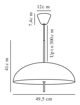
Voltage (V): 220-240 Volt IP degree: IP20
