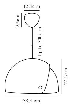
Voltage (V): 220-240 Volt IP degree: IP20 Maximum bulb wattage (W): 15W Class (Class 1, Class 2, Class 3): Class 2 (Double isolated) Socket type: E27
