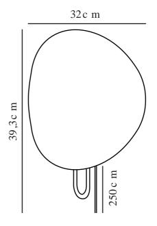
IP degree: IP20 Maximum bulb wattage (W): 25W Class (Class 1, Class 2, Class 3): Class 2 (Double isolated) Socket type: E27
