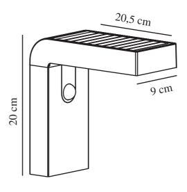
IP degree: IP44 Class (Class 1, Class 2, Class 3): Class 3 (12V) Socket type: SolarLed
