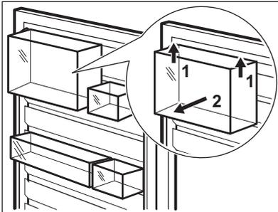
2. Remove the upper rail grabbing and lifting it from the center.
