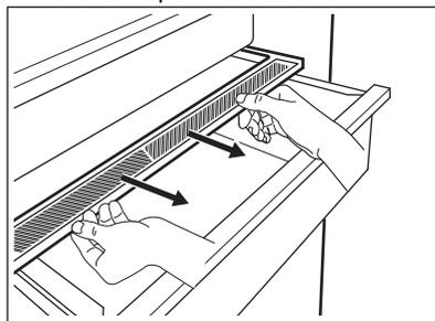
2. If you need to replace the device's white membrane, grab the device in the middle and separate the membrane from the cover by pulling the cover.
