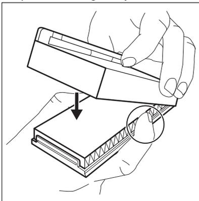
4. Remove the top glass shelf from the fridge compartment. Slip the plastic housing with the air filter on the left side of the glass shelf.
