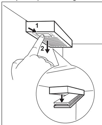
2. Pull out the used air filter.
