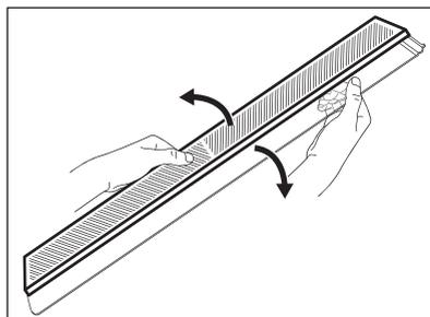
3. Assemble a new membrane into the cover by pressing the edge of the membrane into the cover.
