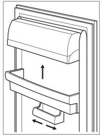
This model is equipped with a variable storage box which can be moved sideways.
