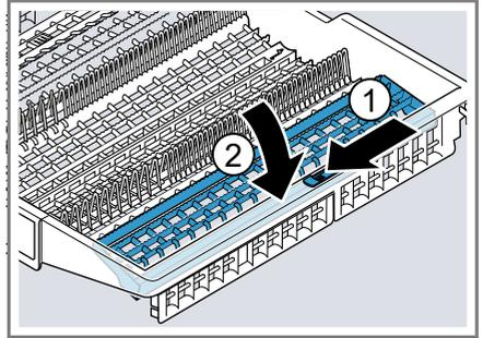
2. To fold down the folding spines, push the lever forwards and fold down the folding spines ①.
