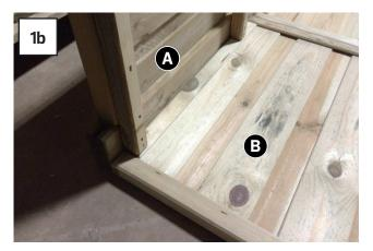
Set out Side Panels (A) and Back Panels (B) as shown in above and fix together using 6 x 60mm Screws – 3 per side.
