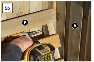
Position Seat Back Rest F between the Side Panels A (Fig.5a). Attach to the Hinged Seat Assembly E using 2 x 60mm Screws – 1per side (Fig.5a) and to the Side Panels A using 2 x 60mm Screws 1per side (Fig.5b)
