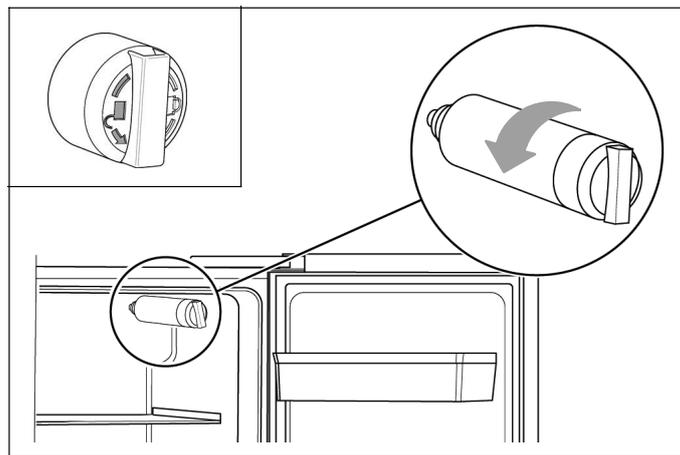
2. Screw out the old water filter in anticlockwise direction (see sign on the filter) and remove it.
