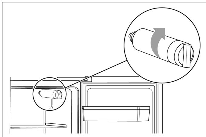
1. Screw in the new water filter in clockwise direction and make sure it is firmly fitted to the water filter base.
