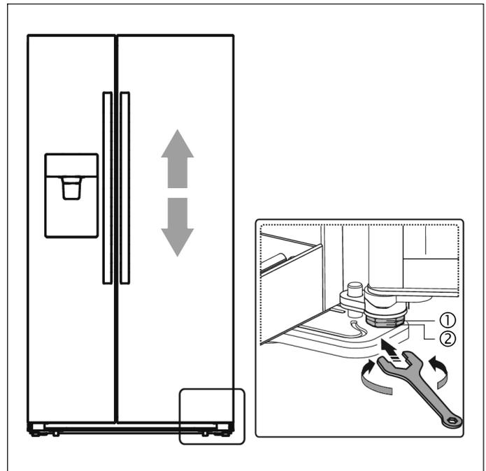
To raise the fridge door, turn the bolt (1) anticlockwise.
