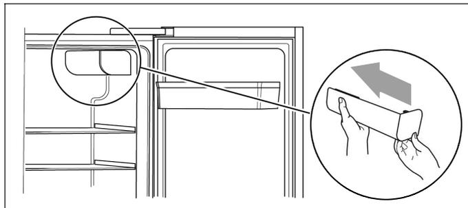
2. Reattach the filter cover by gently sliding it on.
