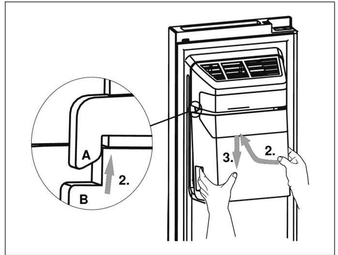
2. Hold at the handle and push up the ice bucket. Ensure that on both sides the ice bucket (B) is wedged into the buckles (A) of the ice maker.
