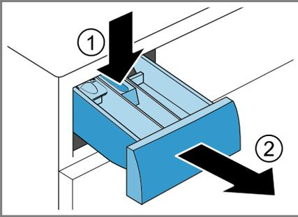
3. Pull out the insert upwards.
