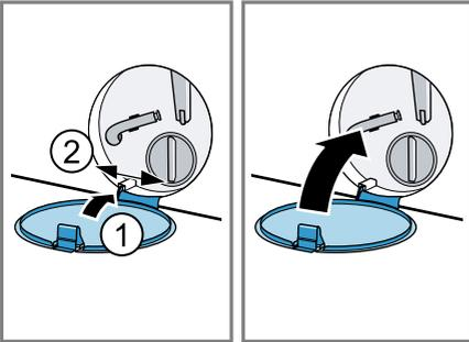
2. Remove any blockages from the intake opening.
