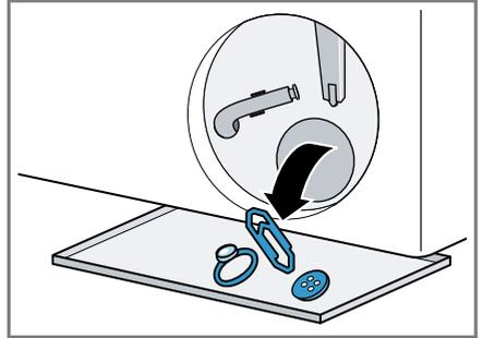
3. Ensure that both impellers can turn.
