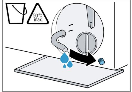
8. Firmly press on the sealing cap.
