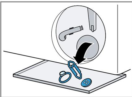
3. Ensure that the impeller in the drain pump can rotate.
