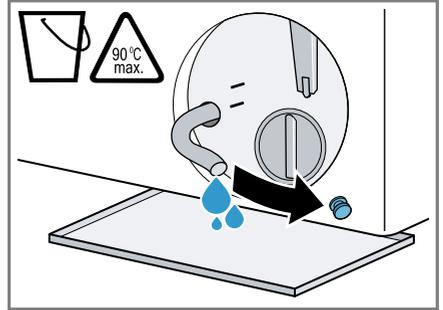
8. Firmly press on the sealing cap.
