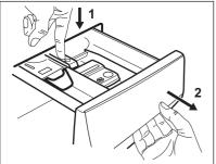
3. To use liquid detergent, adjust the flap in right position, turn the flap down.
