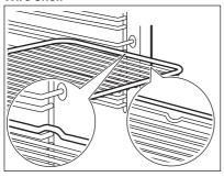
Insert the shelf between the guide bars of the shelf support and make sure that the feet point down.
