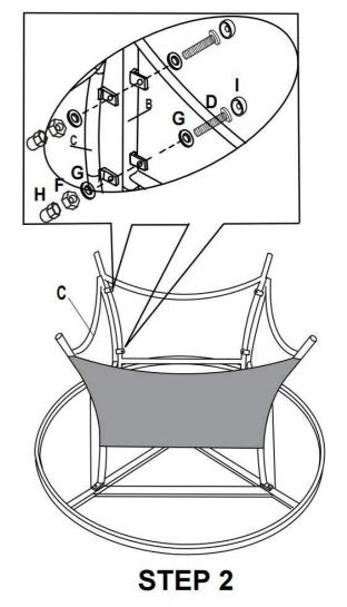
PLEASE ENSURE ALL FIXINGS ARE LEFT LOOSE DURING ASSEMBLY BUT ARE SECURELY TIGHTENED UPON COMPLETION.
