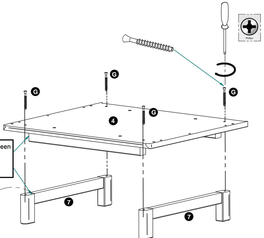
After assembling there might be a small gap between the horizontal rail and the foot of the product. This is intentional to easy assembling and prevent damage to the pieces.
