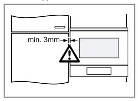
There must be an air gap of at least 3 mm between the appliance and adjacent unit fronts.
