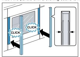
The arrow inside the panels must point upwards. Position the groove on the panels above the corresponding transverse rib on the red fastening part.
