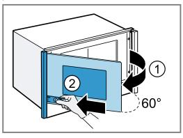
2. To loosen the panel, close the appliance door ① and at the same time press the fastening element on the appliance door down and towards the panel ②.
