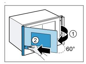
**2.** To loosen the panel, close the appliance door ① and at the same time press the fastening element on the appliance door down and towards the panel (2)
