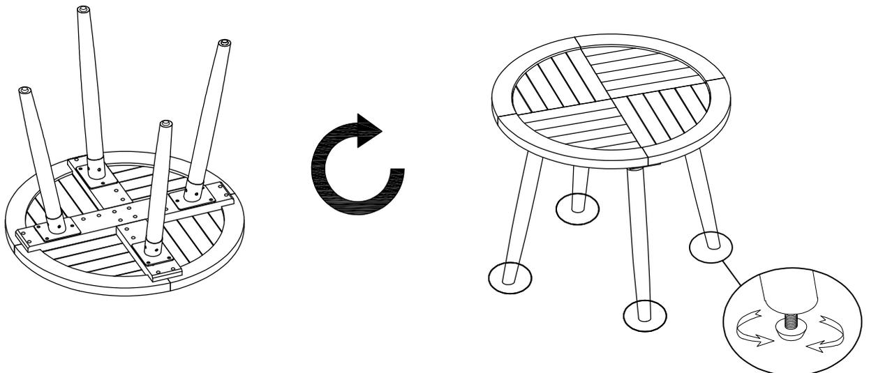
With 2 people, carefully turn and place the table on its feet. Take care when lifting not to damage the legs. Once in position, turn the adjustable feet so it sits flat on the ground.
