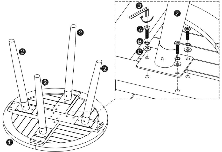
Find a clear area for assembly, near where you intend to use the table. Place table top (1) upside down on a soft surface. Then locate the legs (2) and secure using the Allen bolt (A), Lock washer (B), Washer (C) tightening with the Allen key (D) provided. Repeat this process for all legs
