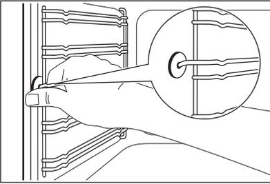
2. Pull the rear end of the shelf support away from the side wall and remove it.
