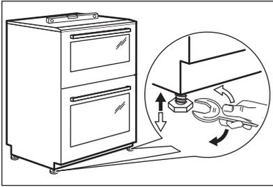
Use small feet on the bottom of appliance to set the appliance top surface level with other surfaces.
