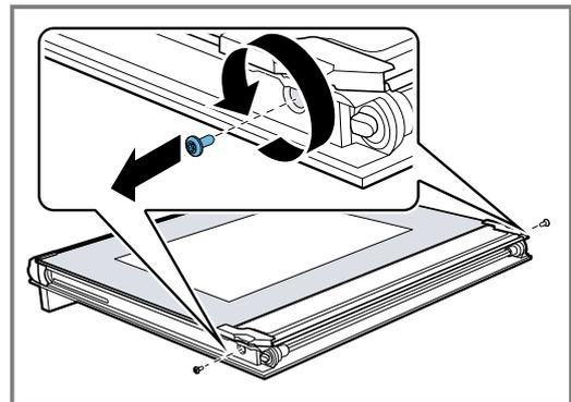
3. Carefully lift the inner pane upwards at an angle ① and remove the holder [a] ②.
