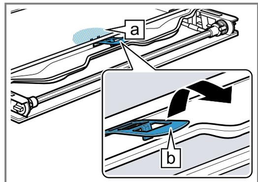
6. Lift the first and second intermediate panes from below ① and remove them in the direction of the arrow ②.
