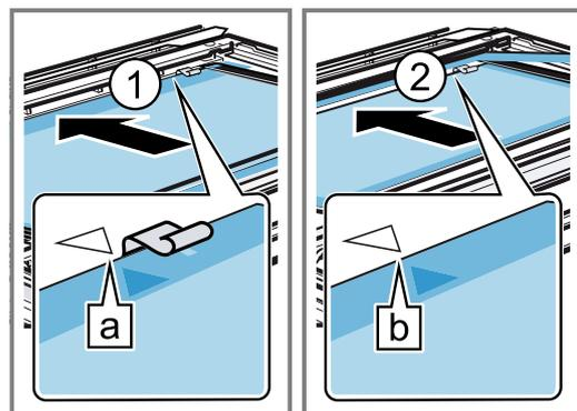
The arrow on the intermediate pane must line up with the arrow on the frame **b**.
