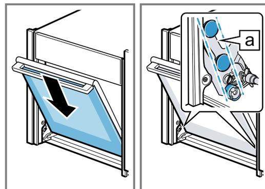
2. Rotate the door handle upwards slightly ①.
