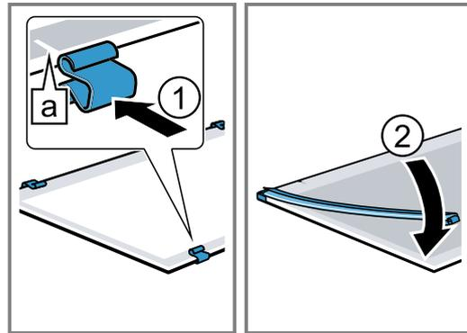
3. Insert the intermediate pane with spacers and seals in the direction of the arrow ①.
