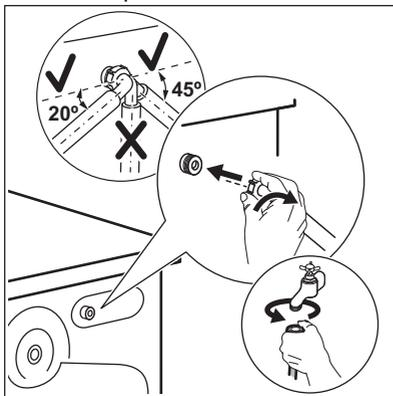
**i** Make sure that the inlet hose is not in vertical position.
