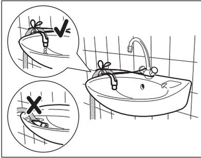
**i** Make sure that the drain hose end is not immersed in the water. There may be a return of dirty water into the appliance.
