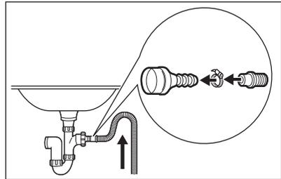
**i** Make sure that the drain hose makes a loop to prevent particles going into the appliance from the sink.
