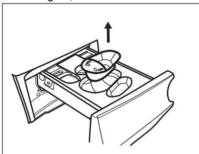
3. Lift up the top cover of the compartments to remove it.
