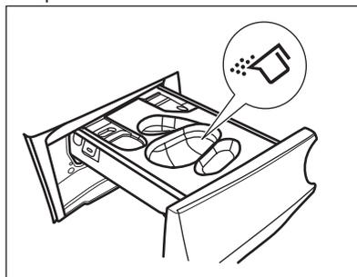
b) Pour the **liquid detergent** in the same compartment after inserting the relevant container
