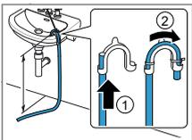
Push the water drain hose fully through the and secure it using fixing material. Secure the elbow at a height of no more than 100 cm.
