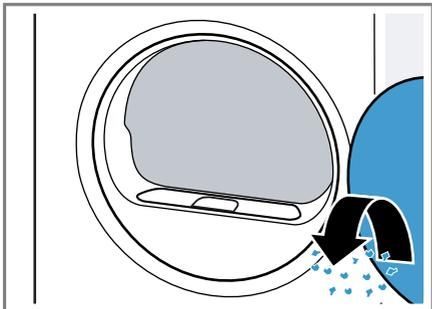
3. Remove the two-part fluff filter.
