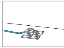
Secure the elbow to the gully.
