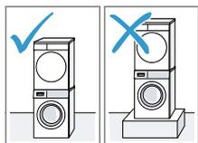
Only use the original connection set from the dryer manufacturer when setting up this appliance in a washer-dryer stack.
