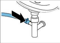
Secure the connection point with a (24–40 mm) hose clamp.
