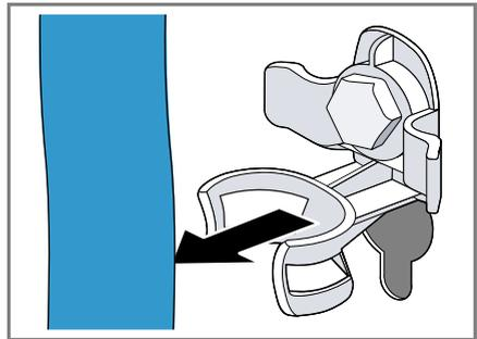
2. Unscrew ① and remove ② all the screws for the 4 transit bolts with a WAF 13 wrench.
