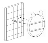
Place hook in desired location and ensure it is level Mark mounting hole locations Drill holes and insert rawl plugs Insert screws into rawl plugs leaving 5mm overhang
