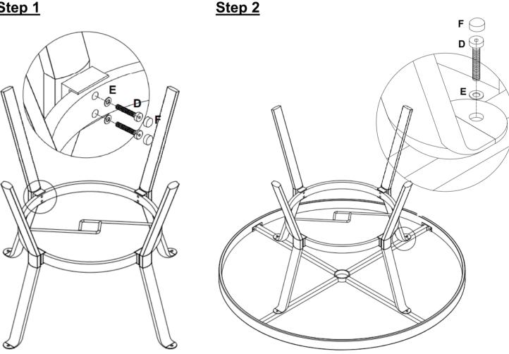
PLEASE ENSURE ALL FIXINGS ARE LEFT LOOSE DURING ASSEMBLY BUT ARE SECURELY TIGHTENED UPON COMPLETION.
