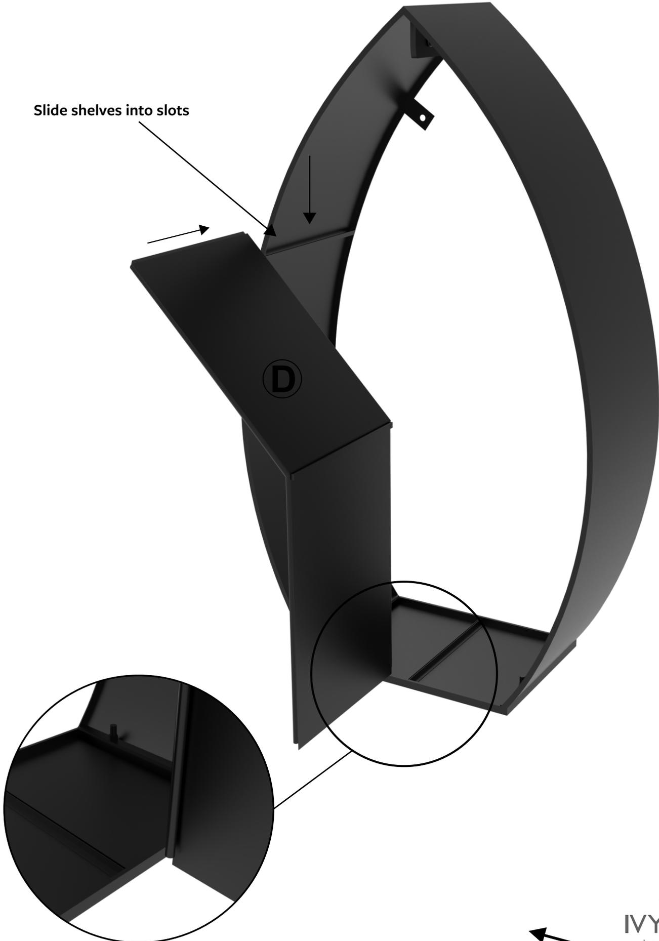
Slide centre piece D into slot at base
