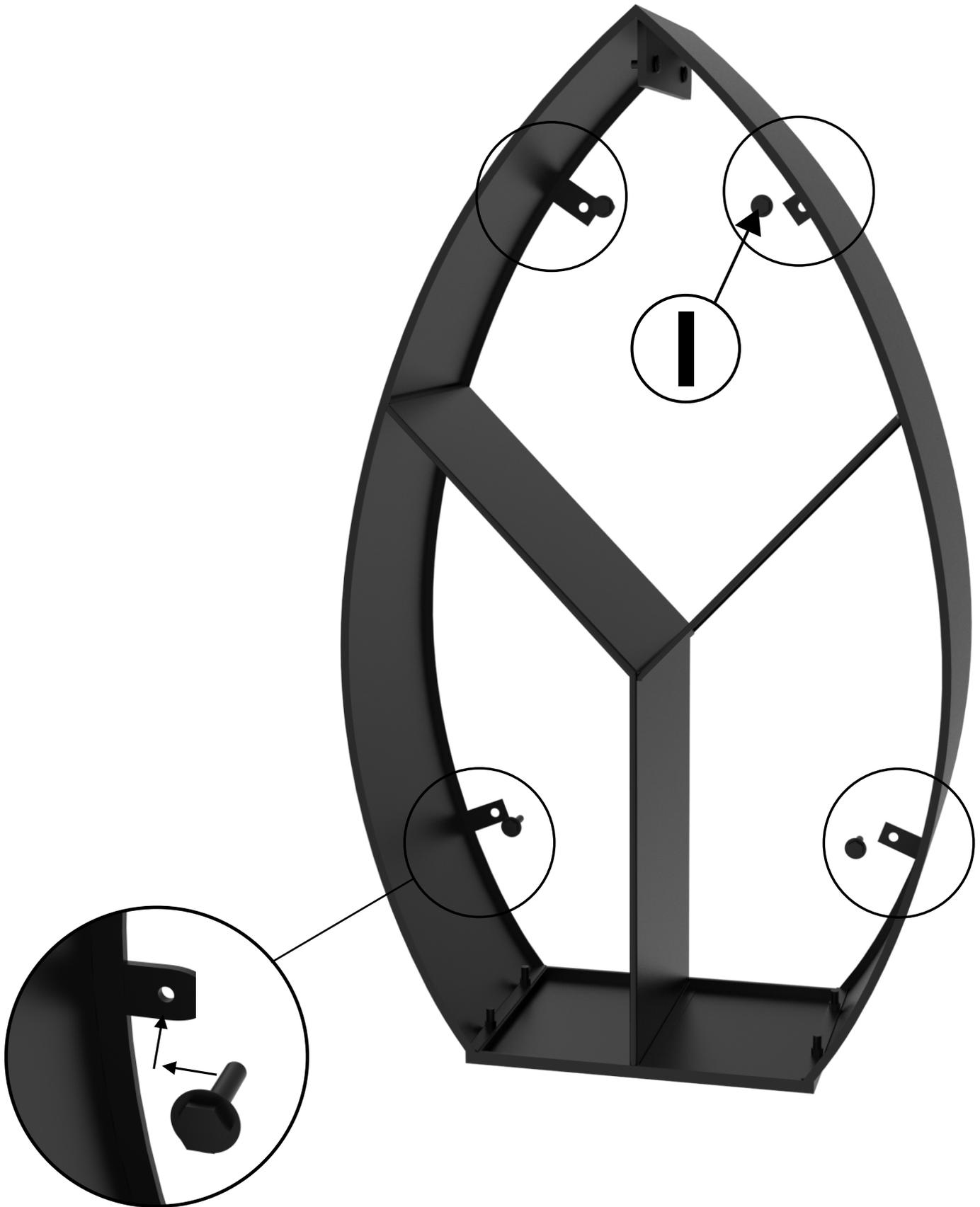
Fix onto the wall with wall fixtures
