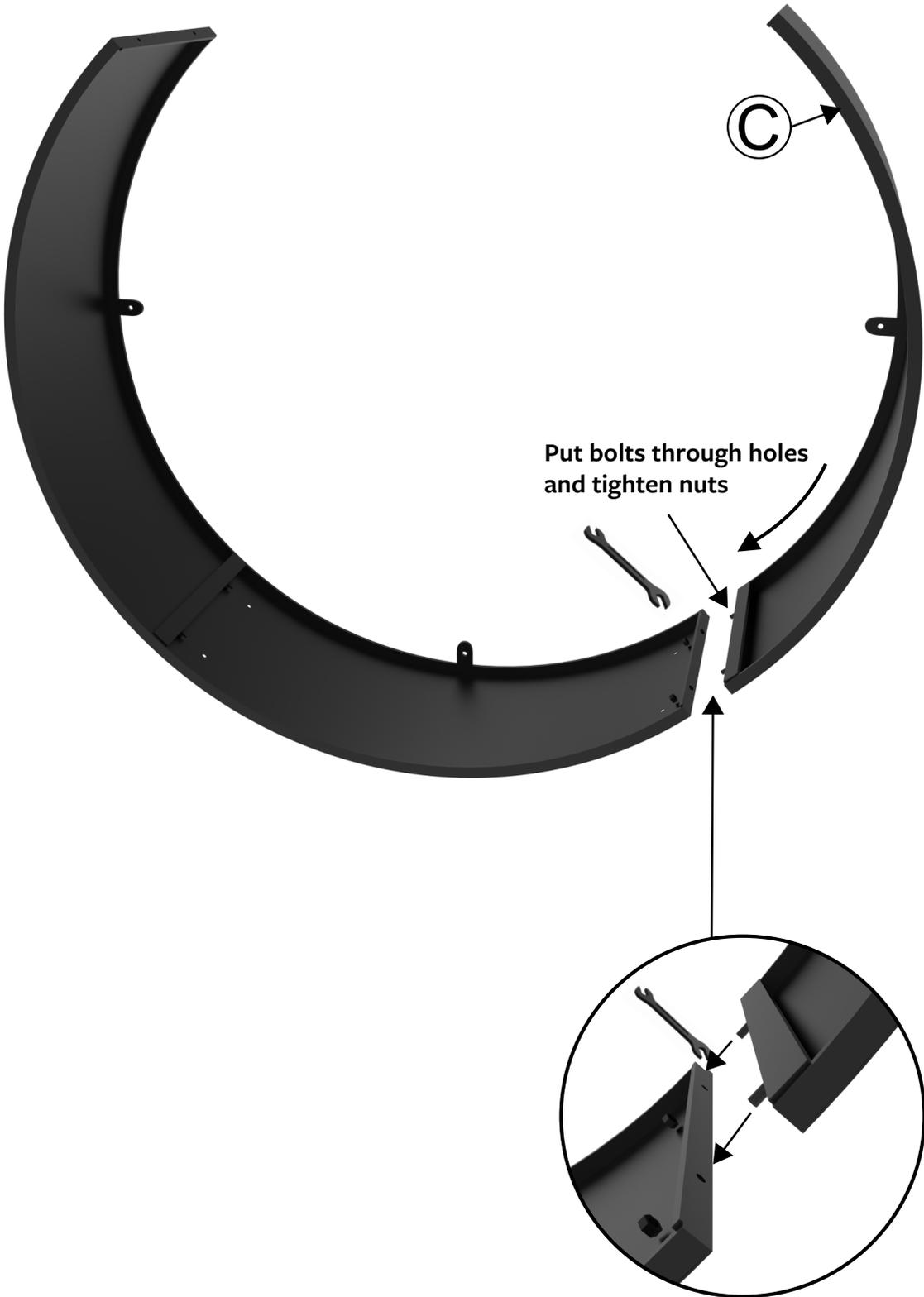
Put bolts through holes and tighten nuts
