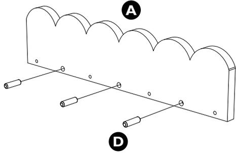
**Step 2** Insert shelf **B** on the dowels **D** then screw in screws **C** through back panel **A**.
