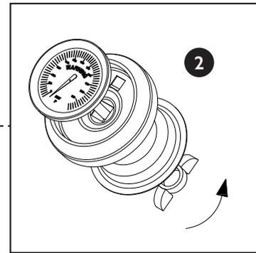
Push Control Knobs (23) onto spindles indicated.
