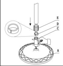
**Step 2:**With A Top upside up, hand (or use bolt driver) tight, put the appropriate size D on the pole, then put E on D
