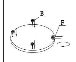
**Step 1:**With A Top upside down, fix B into the bolt holes provided, using F to tight.
