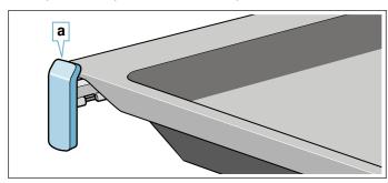
The pull-out rails lock in place when they are fully pulled out. This makes it easy to place the accessories in position. To unlock the pull-out rails, use a little force to push them back into the cooking compartment.
