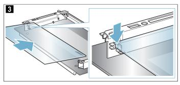
4. Place the outer disc on the seala (Fig. 4).
