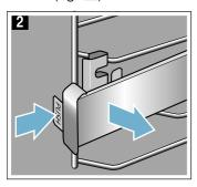
3. Pull the rail out towards you until the retainer at the back unhooks (fig. 3).
