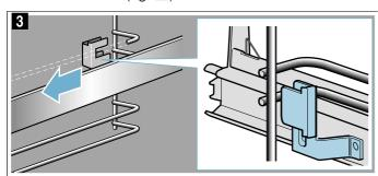
4. Remove the pull-out rail (fig. 4).
