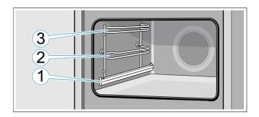
Always insert accessories between the two guide rods for the shelf position.
