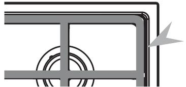
Correct positioning of pan supports (CG604DX models)
