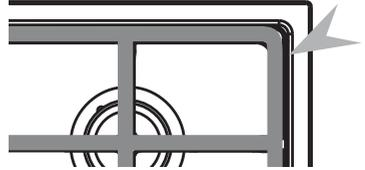
Correct positioning of pan supports (CG905DX models)
