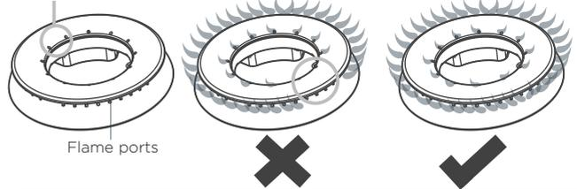
Burner parts may not have been replaced correctly. Check the assembly and make sure the burner cap and/or ring is sitting flat on the flame spreader. See 'Care and cleaning' for illustrations.
