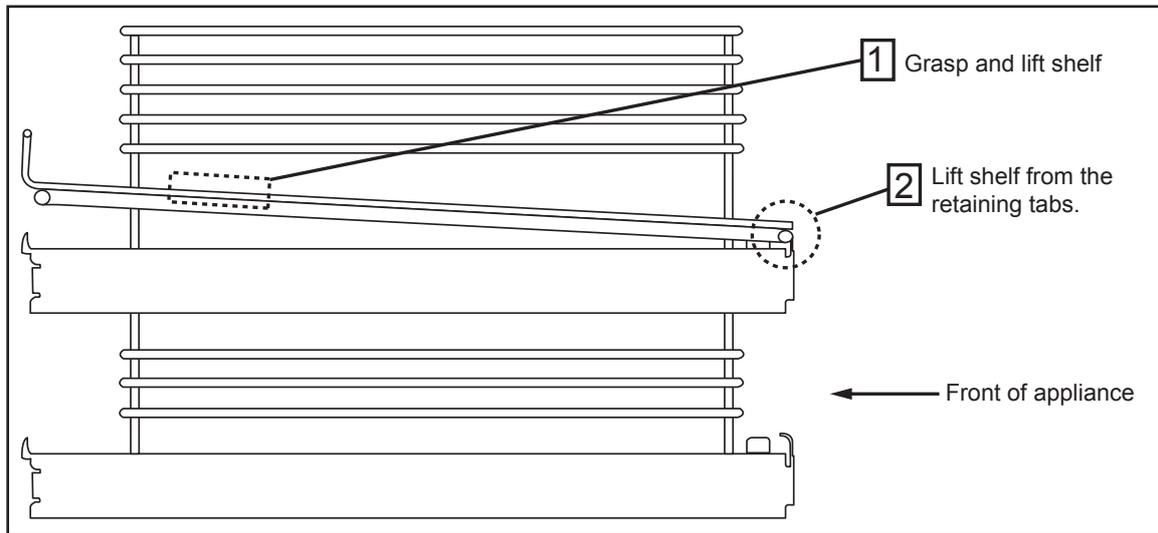
Before removing the shelves completely, please make sure that the shelf is unclipped from the retaining tabs.
