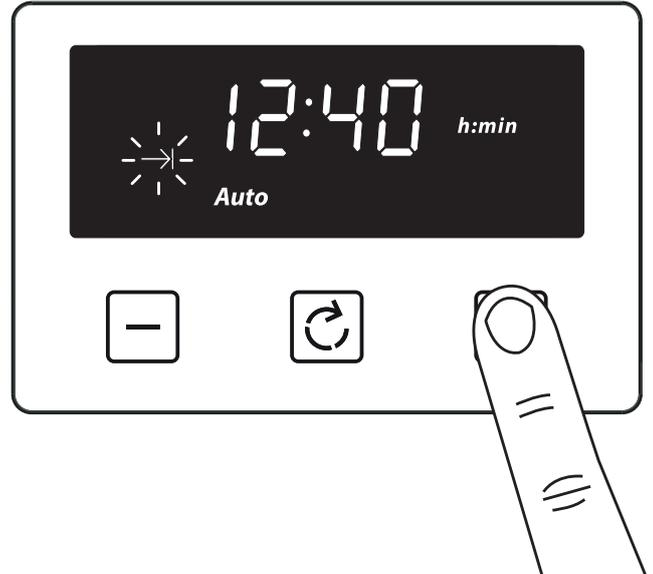
The auto cooking symbol disappears from the display once the time, the required cooking settings and temperature have been set. The appliance will not be switched on until the set cooking start time, that is the difference between the cooking end time and the cooking duration.
