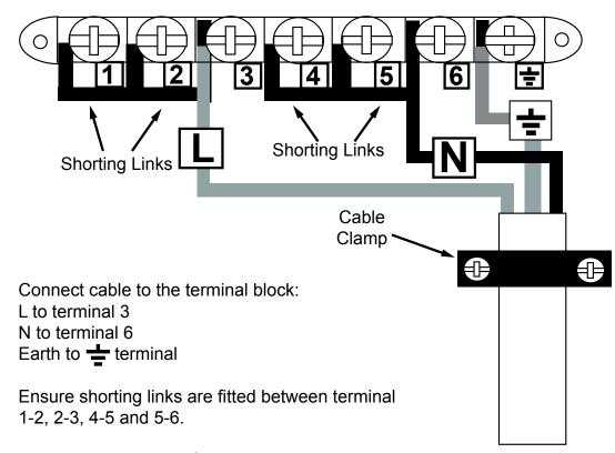
Ensure all screws are fully tightened.
