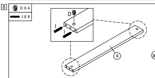
Insert the Large Camfix (D) and Dowels (I) into the pre-drilled holes at either end of the Drawer Slide Support Rail 2 (4) as shown in the diagram. Repeat this step for both Drawer Slide Support Rail (4).
