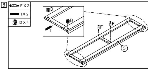
Insert the Dowels (I) and Large Camfix (D) into the pre-drilled holes at each end of the Footboard Frame (5). Next insert the Large Minifix (F) into the pre-drilled holes along the Footboard Frame (5) as shown in the diagram.
