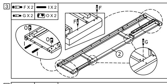
Insert the Large Minifix (F), M8 x 30mm Dowels (I), Barrel Nuts (O) and Small Minifix (G) into the pre-drilled holes on the Right Side Rail (2) as detailed in the diagram.
