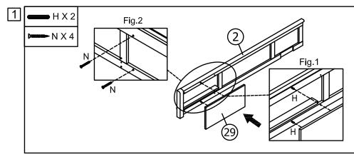
Insert the M6 x 30mm Dowels (H) into the pre-drilled holes along the Right Side Rail (2) as detailed in the diagram. Attach the Side Rail False Drawer (29) to the Right Side Rail (2) and secure in place using M4 x 25mm Screw (N) as shown in Fig.2.
