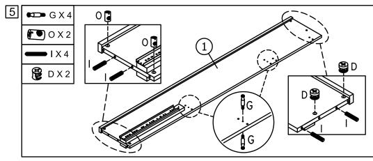
Insert the M8 x 30mm Dowels (I), Large Camfix (D), Small Minifix (G) and Barrel Nuts (O) into the pre-drilled holes on the Centre Frame (1) as detailed in the diagram.
