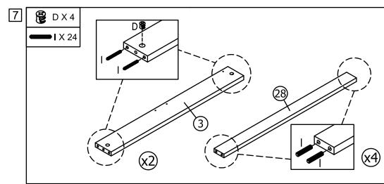
Start by inserting the Dowels (I) and Large Camfix (D) into the pre-drilled holes on each side of the Drawer Slide Support Rail 1 (3). Next insert the Dowels (I) into the pre-drilled holes on each end of the Bottom Rail (28). Repeat this process for both Drawer Slide Support Rail 1 (3) and Bottom Rails (28).
