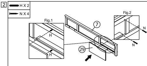
Insert the M6 x 30mm Dowels (H) into the pre-drilled holes along the Left Side Rail (7) as detailed in the diagram. Attach the Side Rail False Drawer (29) to the Left Side Rail (7) and secure in place using M4 x 25mm Screw (N) as shown in Fig.2.
