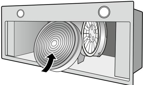
2. Guide the activated charcoal filter around the motor.
