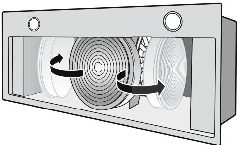
3. Carefully slide the new activated charcoal filter into the retainer.
