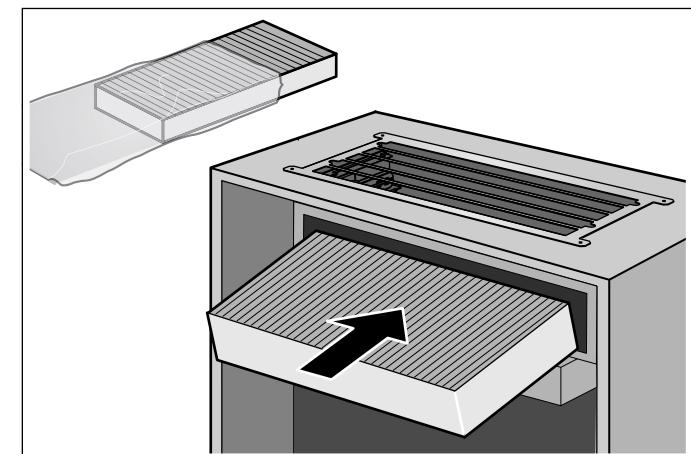
2. Fit the panel such that it is held firmly in place by the magnets.
