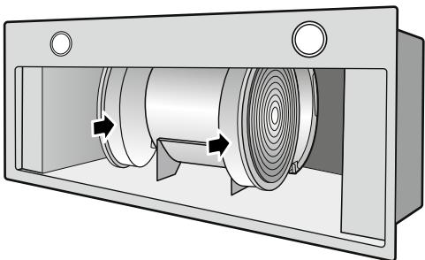
4. Install the metal grease filters.
