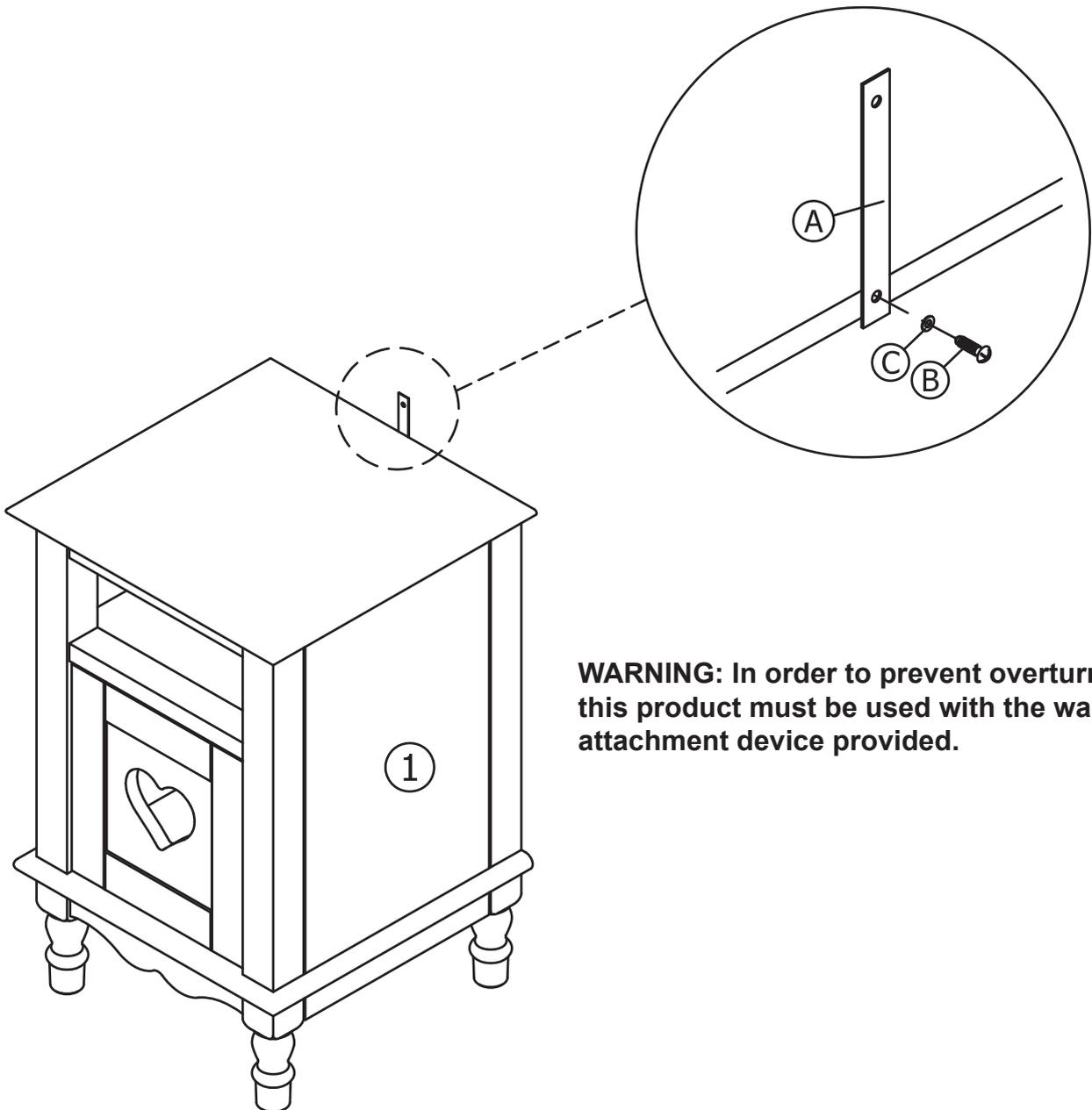
**WARNING:** In order to prevent overturning, this product must be used with the wall attachment device provided.
