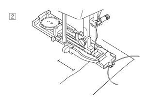
2 Start the machine and sew the buttonhole. Each side of the buttonhole and the bartacks will be sewn over the cord.
