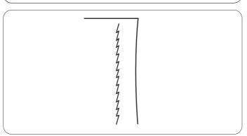
This stitch is a narrow stretch stitch designed to eliminate puckering on knit fabrics and bias seams, while permitting the seam to be pressed completely open flat. Use this stitch for seaming fine fabrics.
