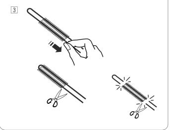
3 Pull the loose ends of the filler cord to tighten it. Cut the both ends of the filler cord.
