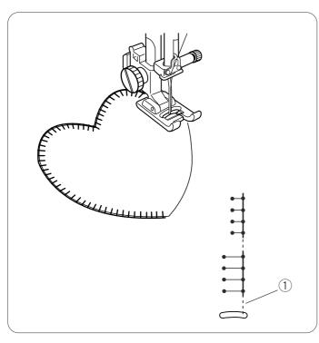
Place an applique on the fabric and baste or pin it in place.
