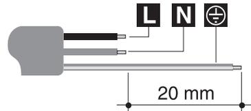
Only use a H05V2V2-F or similar cable resistant to the maximum temperature of  $90^\circ\text{C}$ . The cable must be replaced by a specialised technician who must carry out the connection to the power grid following the diagram below.
